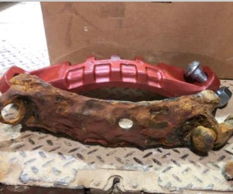
Above Photo: A specialized coupler removed from a waterline on Tracy Road in Northwood, and its custom replacement. Corrosion has caused major damage to several of the rare parts needed to make this repair. We ask for your patience as these unique parts take time for manufacturers to produce.
